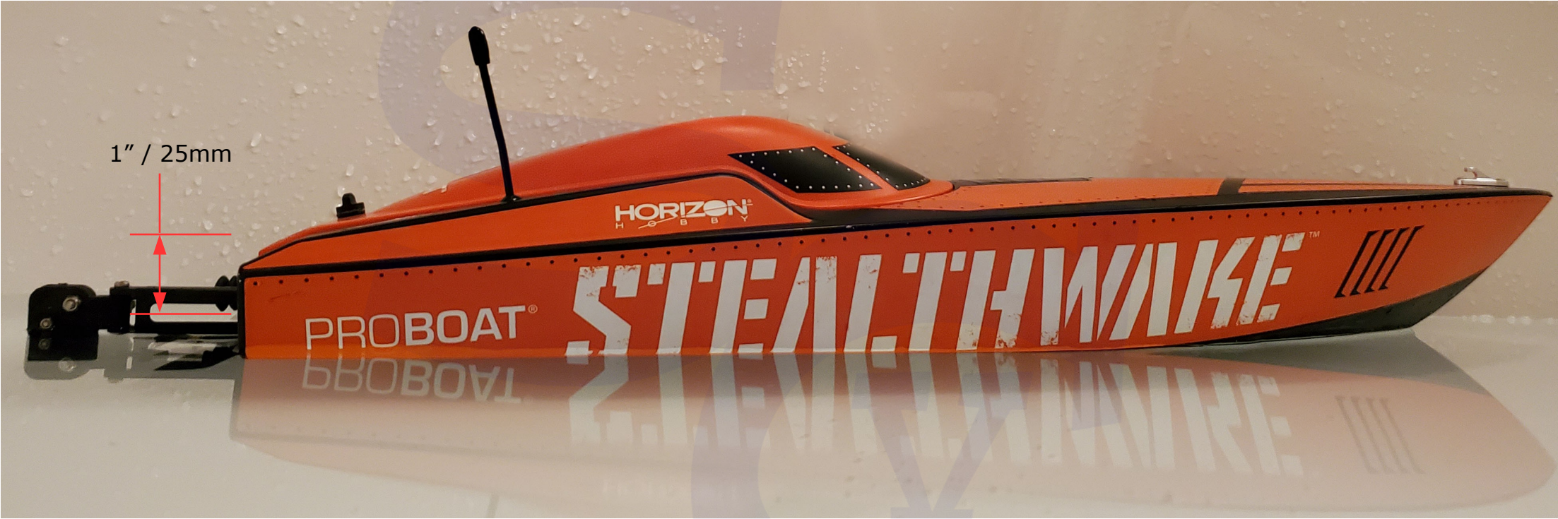
Freeboard: The distance from the waterline to the upper deck level, measured at the lowest point of sheer, where water can enter the boat or ship.
